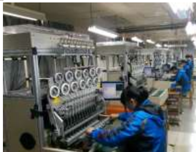
Example of full-auto assembly from winding to termination
