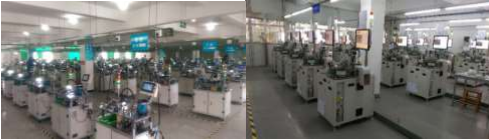
Small toroid winders, typically for LAN products
