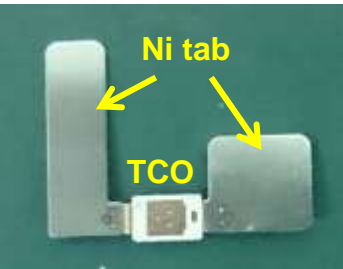
TCO sub Assy (TCO + Ni tab attached by welding)
